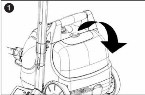
Remove the required steam accessory and replace the cover. Slide the nose of the cover into the recess above the steam socket and press it down firmly at the back until the cover clicks into place.
