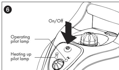
The orange operating light (Fig. 6) lights up and starts heating up the steam cleaner. The operating temperature is reached after about 11 minutes and the green heating pilot lamp lights up. The appliance is now ready for use.
