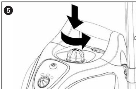
Only fill with pure water without additives of any kind, e.g. perfume, cleaning agents, alcohol, as they could damage the machine and make it dangerous to use. It is advisable to use distilled water to prevent limescale deposits if the water is very hard (above 2.5 mmol/l or 21 °dH). Otherwise, boil the water first to prolong the service life of the appliance.
